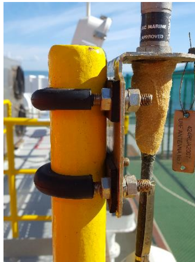
Figure 2: Insulation to avoid galvanic corrosion.
